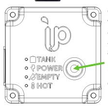
Once a power connection is made, the SolarPlex SPX-800-5 will automatically start in its default MPPT mode, operating at the maximum power available from the connected PV array or power supply up to a maximum rated power of 800W. To **stop and start** the pump, short-press the control button indicated (for up to 2 seconds). For further information on alternative operating modes and LED light display information, refer to sections 9 & 10.
