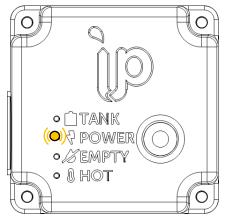
Input power too low. The POWER LED light will flash amber once every two seconds. All other LED lights will be off. This may indicate that the maximum-power voltage (Vmp) of the PV array or power supply is too low or that sunlight levels are too low for your pump to operate.
