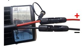
The open-circuit PV panel voltage (Voc) should be less than 105V. For maximum pump power, the PV panel maximum power voltage (Vmp) should be greater than 72V under standard test conditions, i.e. a PV panel temperature of 25 °C.
