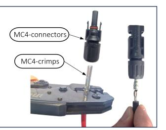
**6** Connect the PV panels to the pump with the MC4-connectors
