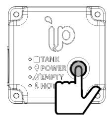
When stopped, 1 short-press (up to 2 seconds) will start the pump. It will start in its default 800W Maximum Power mode unless a power limited mode has previously been selected and saved to memory. In this mode, the POWER LED light will show constant blue.
