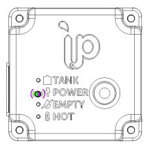
Error codes shown by intermittent green and purple flashes of the ONDER LED light are not user serviceable. Nonetheless, they may indicate faulty data communications, if relevant. If any LED colour or flashing codes appear which are not listed here, please make a careful note of which LED is showing an error warning, their colour and the flashing sequence of the warning including the duration of any flashes
