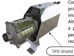
Consider providing shading, for example by installing the protective SolarPlex Shield (SPX-Shield) shown in the image on the left which is available from your distributor. Alternatively, move the pump to a cooler location or select a power limited mode (see section 9). If the problem persists, disconnect power, wait several minutes and reconnect.
