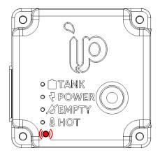
Input voltage TOO HIGH The light will fast-flash red, on and off for equal durations, two times every second. This may indicate that the open-circuit voltage (Voc) of the PV array or power supply is too high. Immediately isolate or disconnect to avoid damage to equipment and refer to section 6 of this guide.
